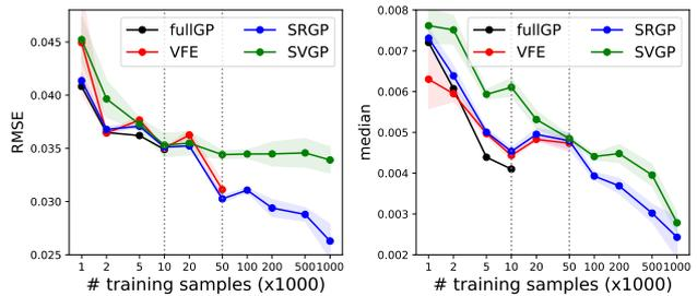
Fig. 9. RMSE and median for full GP, batch sparse GP (VFE), sequential SVGP, and our recursive method (SRGP) trained on varying time horizons (logarithmic scale). The grey dotted vertical lines at  $10'000$  and  $50'000$  indicate the maximal samples used for training full GP and sparse batch GP (VFE), respectively.
