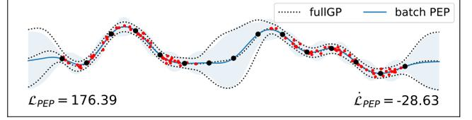
Fig. 1. Full GP and batch sparse GP regression with PEP model ( $\alpha = 0.5$ ).  $N = 100$  data samples are summarized with 15 equidistant inducing points (black dots). A slightly smaller than optimal lengthscale was selected and no parameters  $\theta$  were optimized. The numbers in the left and right corner indicate the lower bound to the log marginal likelihood in (4) and its derivative with respect to the lengthscale, respectively.
